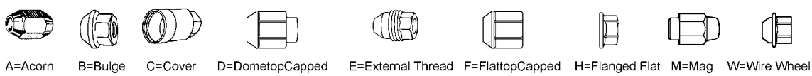
A=Acorn B=Bulge C=Cover D=DometopCapped E=External Thread F=FlattopCapped H=Flanged Flat M=Mag W=Wire Wheel S=Standard
