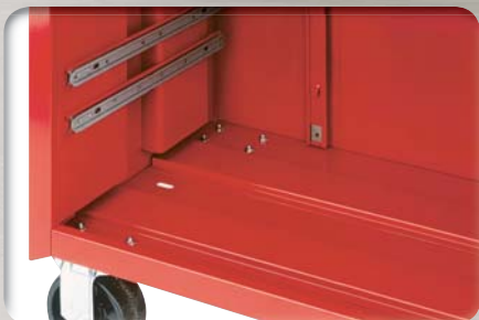
"C"-Channel Base - Double "C"-Channel reinforcement on inside of bottom on roller cabinets increases load bearing capacity by over 30%. "C"-Channel also keeps box rigid and square.
